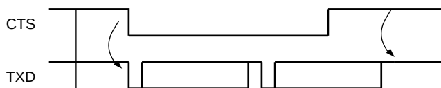
Figure 32-29. Transmitter Behavior when Operating with Hardware Handshaking
